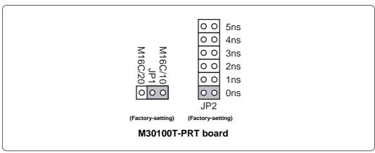
Figure 4.3 Switch settings (factory-settings) for the self-check
